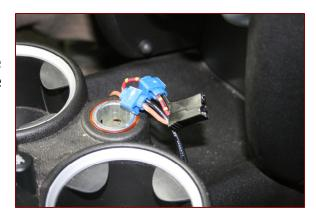
positive wire, and the car's ground wire is the plain brown wire. Connect the red and green striped wire to the extension wire with red marking, and then connect the two plain wires, using the supplied taps.
